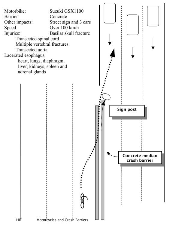
The rider attempted to turn left from the inside lane of a two-lane approach to a Tintersection. Turning sharply left at excessive speed before a divider for the inside and outside lanes the rider lost control and impacted the crash barrier on the opposite side of the intersection at an angle of roughly 75 degrees
