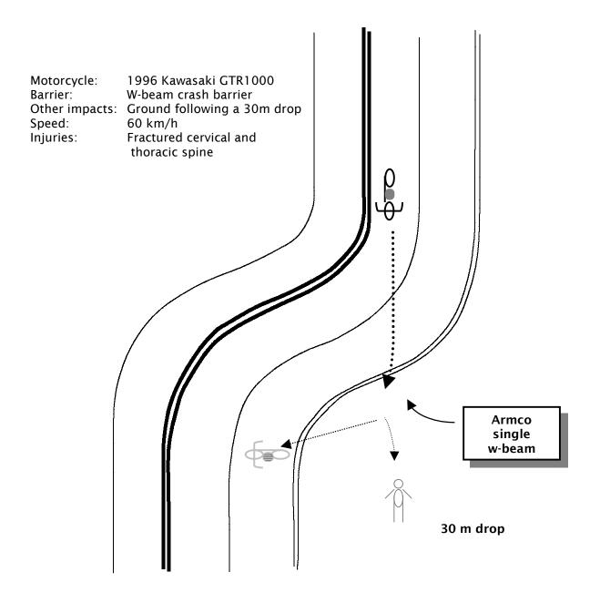
The motorcycle rider ran off the left-hand side of the road into a crash barrier on the outside of a right hand bend. In this case the rider fell on to their right side and slid into the crash barrier at an angle of approximately 45 degrees. The front of the rider's helmet collided with a crash barrier post causing severe neck and spinal injuries.
