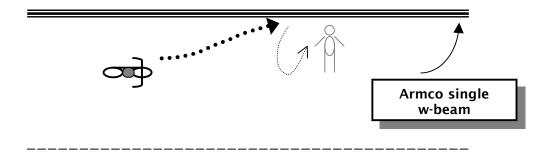
This crash occurred with a crash barrier in a metropolitan area. The rider impacted a w-beam crash barrier at approximately 45 degrees and an estimated speed of 60km/h after failing to take a sharp right hand bend. The motorcycle, a Kawasaki GTR1000 bounced back into the lane and the rider was launched over the crash barrier and down a 30m drop. The main injuries found were severe neck and chest injuries with fractures of the cervical and thoracic spine.
